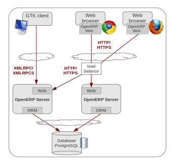
Fig. 1.1: OpenERP 6.1 architecture for embedded web deployment
